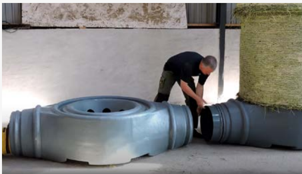
Mounting and connection of the modules can be done without tools.
